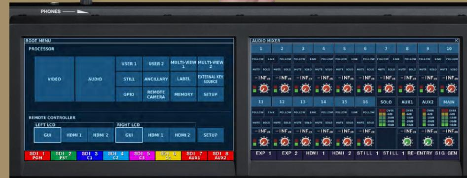
All functions and setting changes are accessible from the root menu. This instantly calls up the required operation screen from among the large number of parameters. These operations can be performed not only via the dedicated
