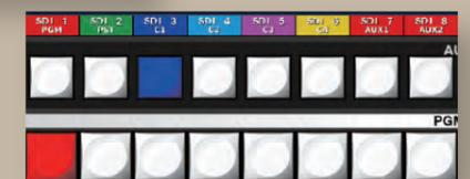
Primary inputs are freely assignable to any cross-point location. Quick input changes can be accommodated easily because the source labels follow simultaneously.
