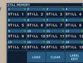
Up to 16 still-images in BMP or PNG format can be stored in the internal memory. The unit supports resolutions up to 1920x1080, and also supports alpha channel for images in PNG format.
