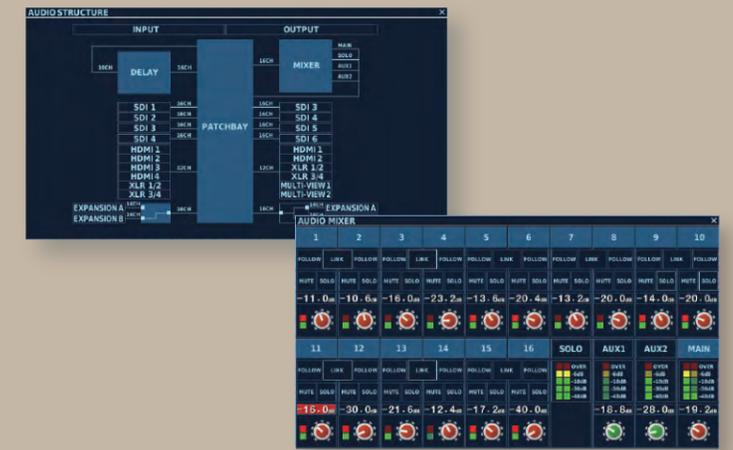
Input and output of up to 92 channels of audio embedded in SDI and HDMI signals is possible. Full 16-channel support is provided for SDI audio. A 16-channel audio mixer equipped with EQ, reverb, and delay is also built-in. Powerful patchbay functionality lets you select 16 sources to be assigned to the audio mixer and also accomplish central control of source feeds as a hub not just for video, but for audio as well.
