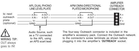
Mountable on 25mm surface back boxes. Outreach plates can be located at any convenient point on an installation, overcoming the need for excessively long microphone or audio leads.
