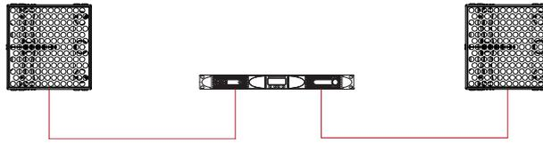
Figure 5.6: 2 x Nexus XL: 8  $\Omega$  per channel/1 amplifier
