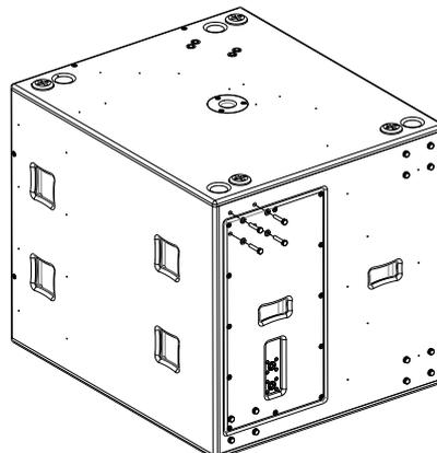
Figure 6.3: Bolt tightening
