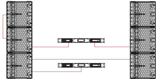
Figure 5.8: 6 x Nexus XL: 8  $\Omega$  per channel/2 amplifier
