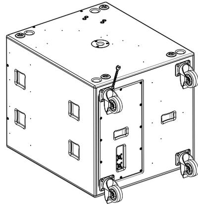
Figure 6.1: Bolt removal
