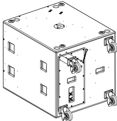
Figure 6.2: Wheel removal
