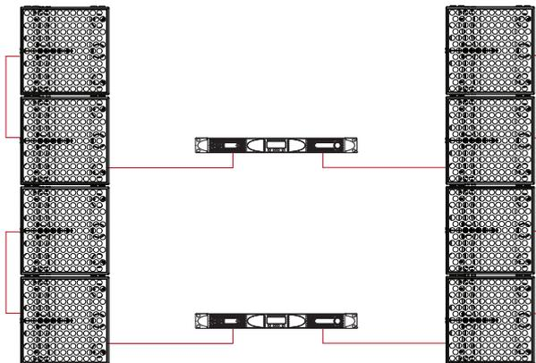
Figure 5.9: 8 x Nexus XL: 4  $\Omega$  per channel/2 amplifier
