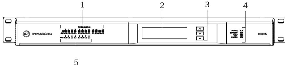
1. Audio inputs 1-12 metering (green = signal present, red = clip) and phantom power (+48 V) indication
