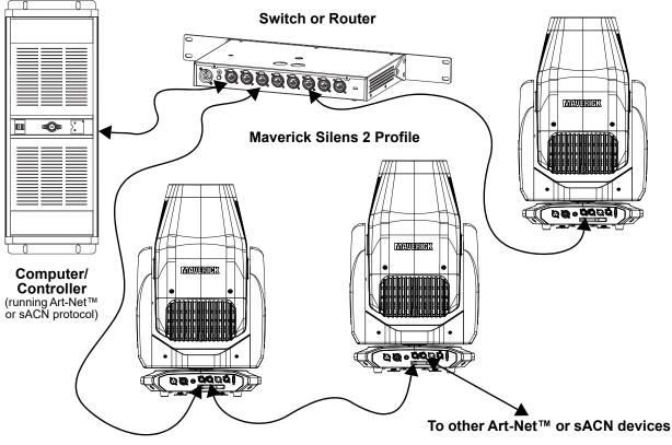
The three LED indicators in between the Ethernet through ports indicate a connection to a network and activity on that network. They do not indicate whether or not the Maverick Silens 2 Profile is receiving a signal from a controller.
