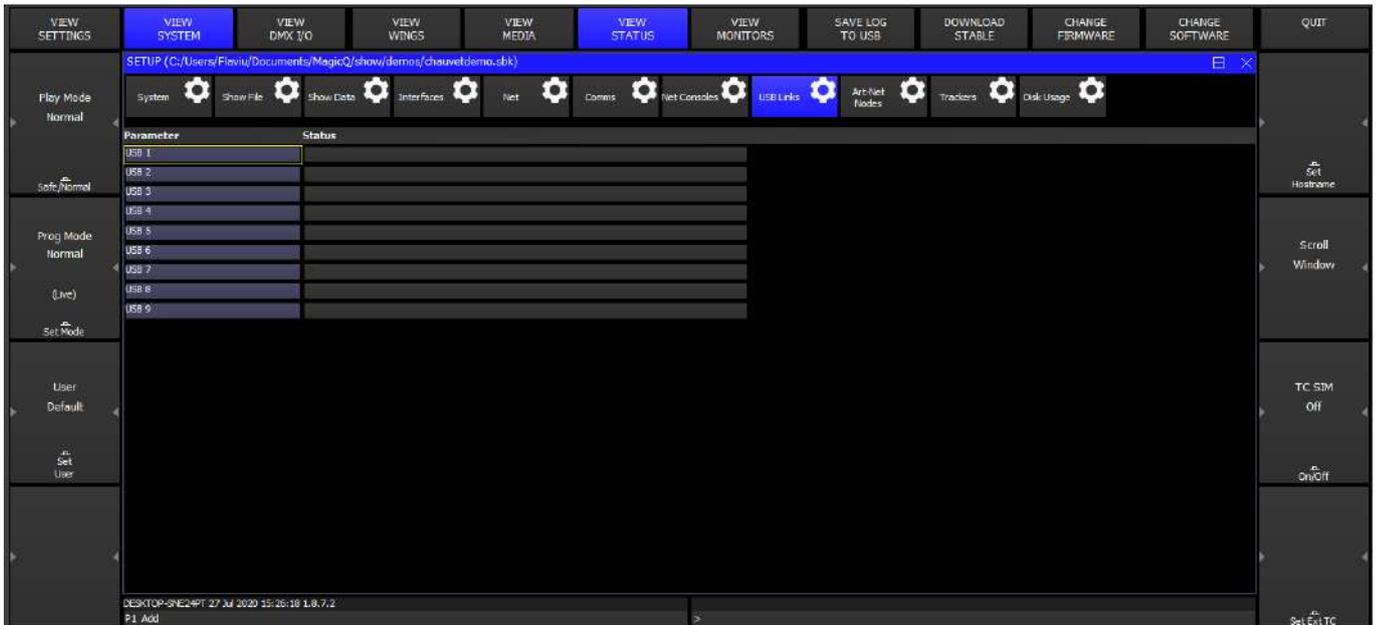
Put the cursor on the line for USB 1 as above. Press CHANGE FIRMWARE and select the new firmware file - e.g. CH331\_V1.0.hex. MagicQ should then say "Starting firmware upgrade" and then a few seconds later "Sent start upgrade".
