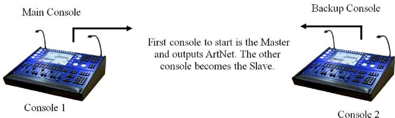
In "Equal mode" all consoles on the network are set to "Hot take-over". At any one time, one of the consoles will run as the master, with all universes enabled. If that console fails, one of the others will take over. It is recommended that you set the "Hot take-over detect time" to different values on each of the consoles to avoid conflict conditions.
