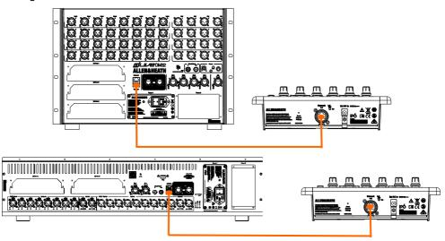
Power up the IP6 by plugging the external PSU into the DC In socket. The port Lnk/Err indicator flashes at a steady rate when the link is established. The unit Name and IP address are displayed on the LCD Displays for easy identification of the unit. After a few seconds the IP6 will display the assignments and functions if any have been set for the unit.
