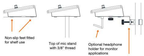
The following accessories can be used to mount the IP6:
