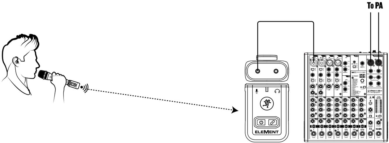
In this example, a Mackie EM-89D mic is connected to the EleMent Wave XLR transmitter. It is paired with its mate, the EleMent Wave receiver. An 1/8" cable is connected between the main output of the receiver and an open channel input of a mixer; a ProFX10v3 mixer, in this case. Then connect cables from the mixer's main outs to the PA system. It is the perfect setup for vocalists with great stage presence who like to roam the stage, presenters who don't want to be tethered by a cable and more!
