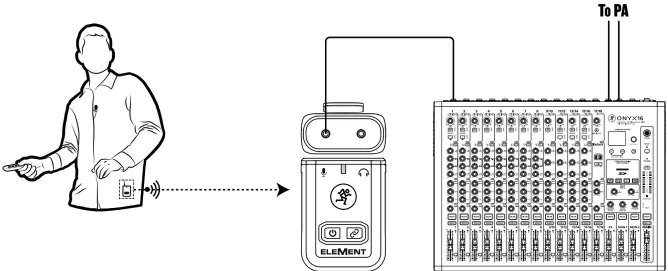
Next up is a look at the EleMent Wave LAV transmitter. You can see here that this is the perfect solution for a hands-free situation. For a more stealth-like presentation, the transmitter is located in the presenter's pocket while the included lav mic (with clip and furry windshield) is clipped to his shirt\*. Now the presenter is free to use a remote control to switch between Power Point™ slides with ease. Or put the remote in the other pocket and break into dance. The world's your oyster!
