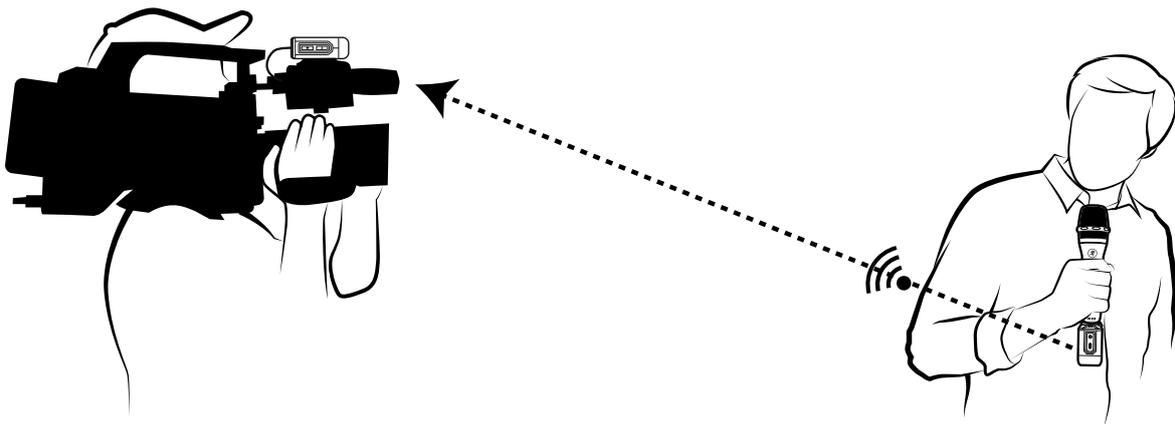
Here's another example that incorporates using a Mackie EM-89D mic that's connected to the EleMent Wave XLR transmitter. It is paired with its mate, the EleMent Wave receiver. As seen above, the belt clip of the receiver may be cold-shoe mounted to a video camera, camcorder or DSLR camera. Then an 1/8" cable is connected between the main output of the receiver and the input of the video camera. This is essentially the exact same type of setup that newscasters use.
