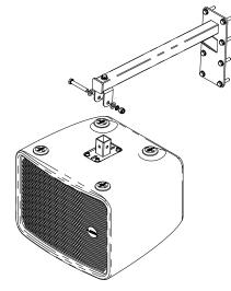
Figure 8.27: Loudspeaker fixing
