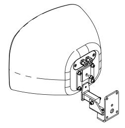
Figure 8.5: Attaching loudspeaker to bracket
