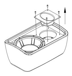
Figure 8.19: Removing horn screws
