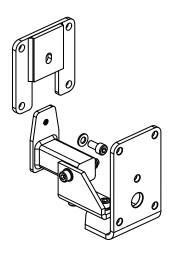
Figure 8.3: Deconstructing the bracket assembly
