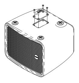
Figure 8.25: Bolt removal
