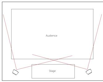
Figure 7.8: Correct horizontal dispersion
