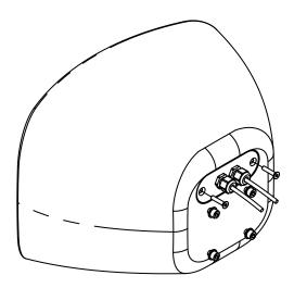
Figure 6.6: Connector plate connection
