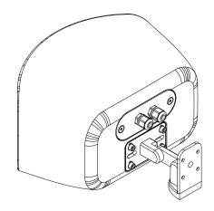
Figure 8.15: Attaching bracket to loudspeaker
