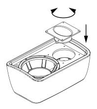
Figure 8.20: Rotating horn
