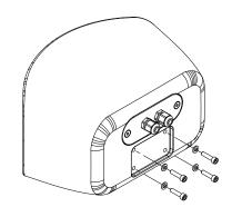
Figure 8.13: Cyclone bolt removal
