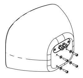
Figure 8.8: Cyclone bolt removal
