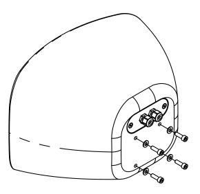
Figure 8.2: Cyclone 8 bolt removal
