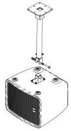
Figure 8.33: Loudspeaker fixing
