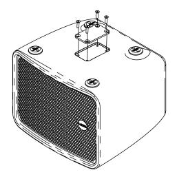
Figure 8.32: Attaching the type 75 plate
