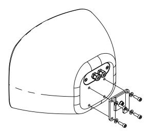
Figure 8.4: Attaching bracket to loudspeaker
