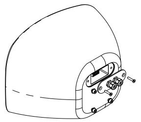
Figure 6.2: Connector plate removal
