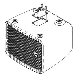
Figure 8.31: Bolt removal
