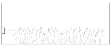
Figure 7.10: Incorrect loudspeaker placement
