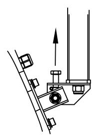
Figure 8.10: Attaching bracket to loudspeaker
