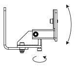
Figure 8.6b: Bracket adjustment
