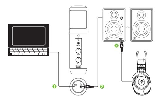
The **EM-USB** microphone is connected directly via USB-C (1) to your computer, for a full computer setup guide, make sure to dive into the **EM-USB** manual.
