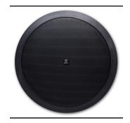
CMX20T two-way built-in loudspeaker produces a warm and deep sound ideal for speech and music. The CMX20T loudspeaker has an 8" enforced polypropylene woofer and 1" tweeter. Due to this enforced woofer, the loudspeaker has a very low distortion! It makes the CMX20T very suitable for the distribution of microphone calls and background music at a higher volume level.
