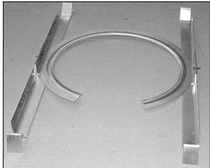
C8.1T rail orientation (rails placed inwards)
