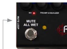
MUTE/LOOP MODE CONTROL ON SIDE PANEL
