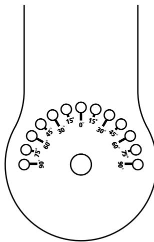
The holes on the bracket allow the speaker to be tilted up to 90° on both sides.
