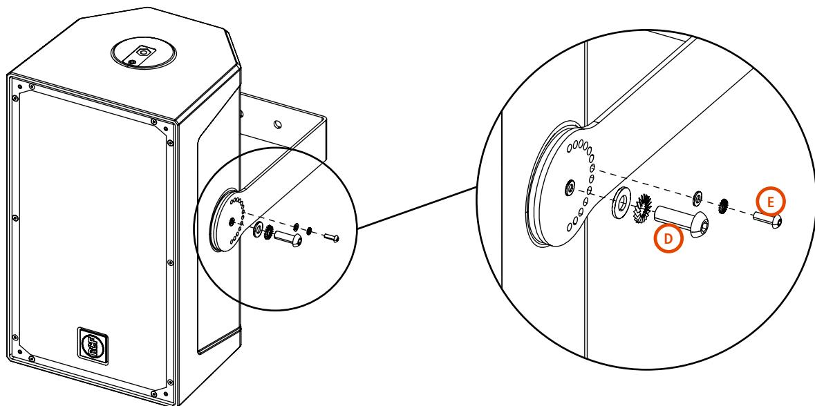
3. Screw the central M10 screw **D** (with its washers) and screw the M5 screw **E** (with its washers) to choose the right angle.
