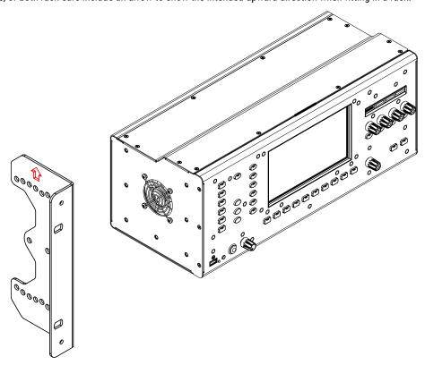
This mounts the SQ-Rack a few millimetres higher in the rack and is only important when rack mounting with the feet already fitted, directly above another unit.
