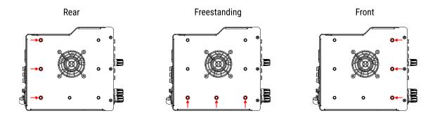
Flush or recessed positions are available when mounting straight  $(0^{\circ})$ , with the rack strip or surface parallel to the front, rear or base of the SQ-Rack.
