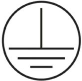
**PROTECTION CLASS 1-FIXTURE MUST BE PROPERLY GROUNDED.**
