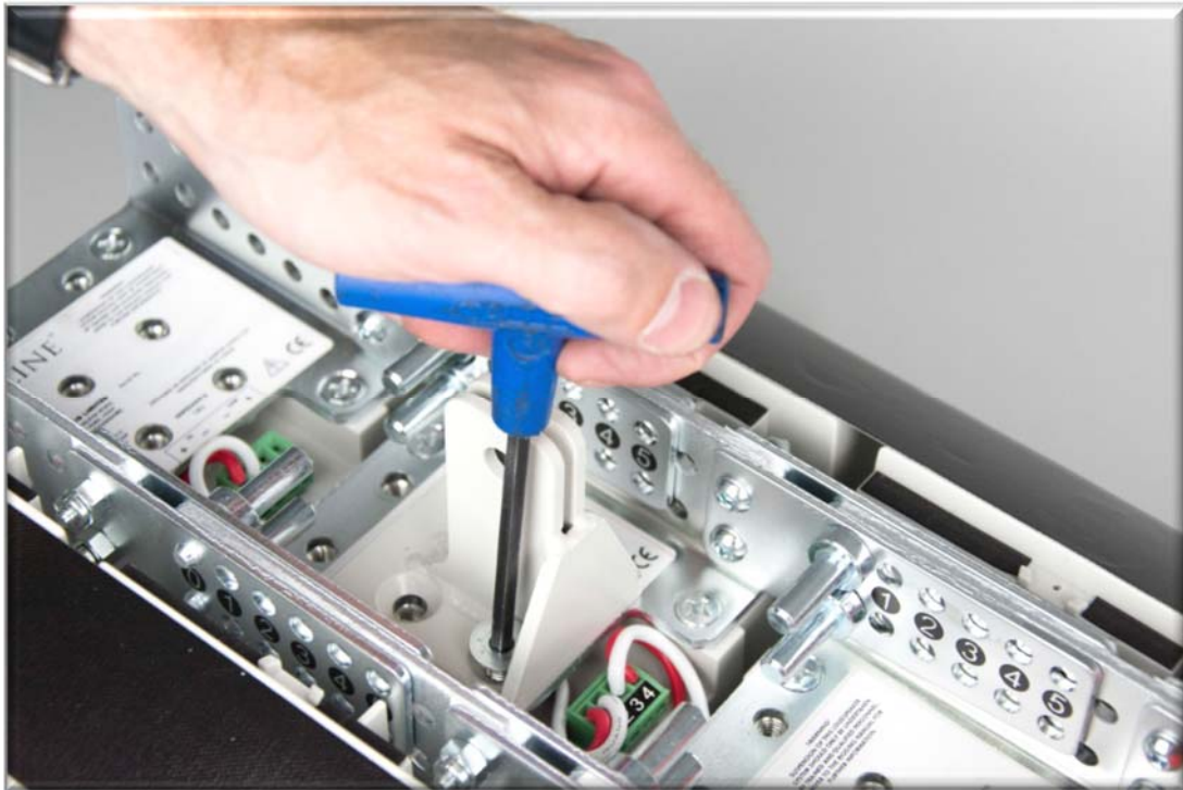
HAM03192 tie bracket in place
