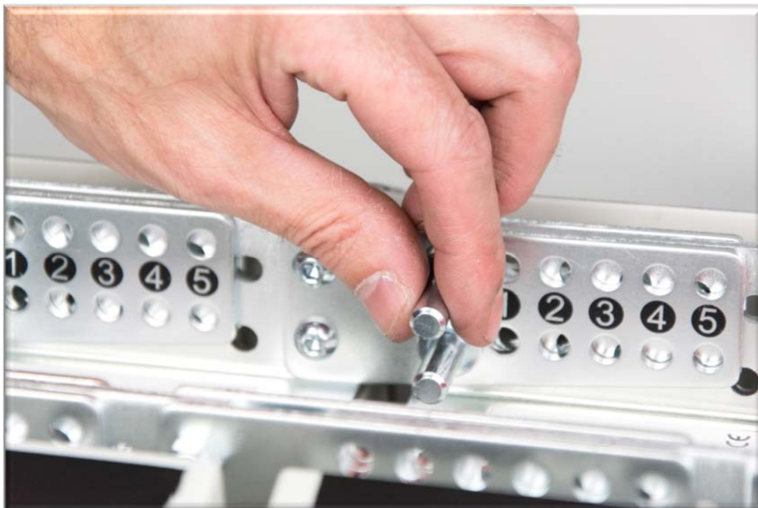
Adding the linking pins
