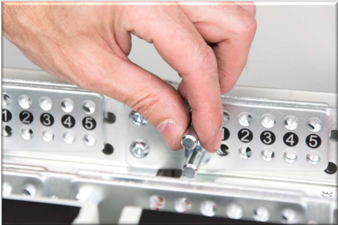
Adding the linking pins
