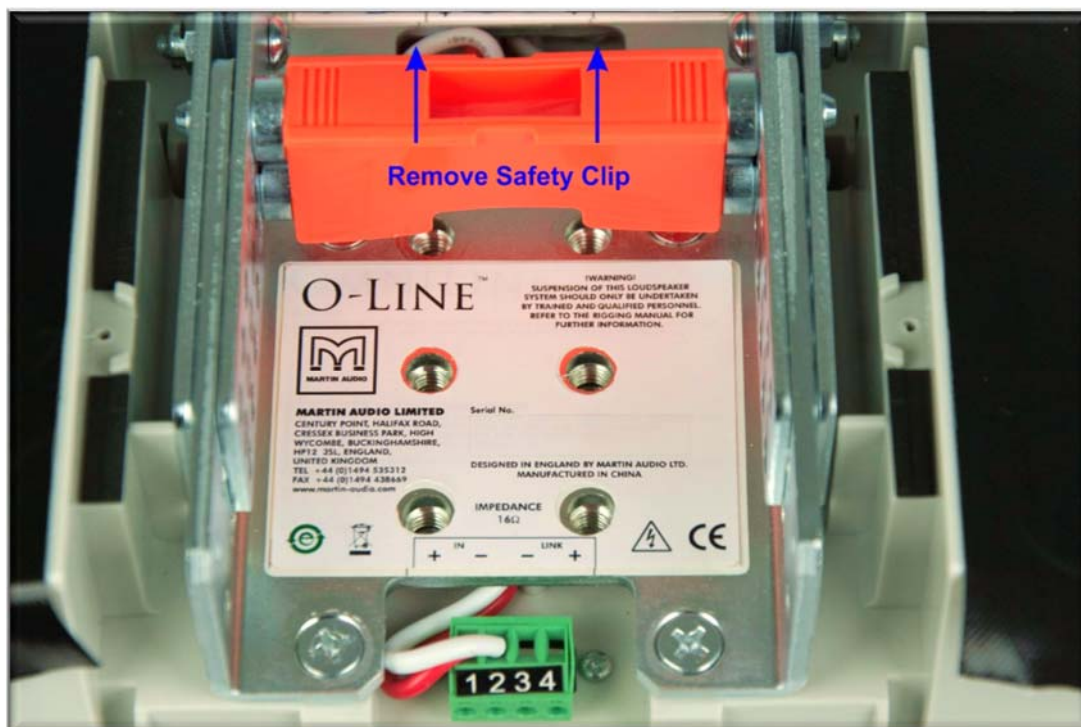
Remove the orange safety clip
