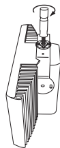
Figure 5.5: Attaching the stud of a floor stand to the suspension bracket of the radiator
