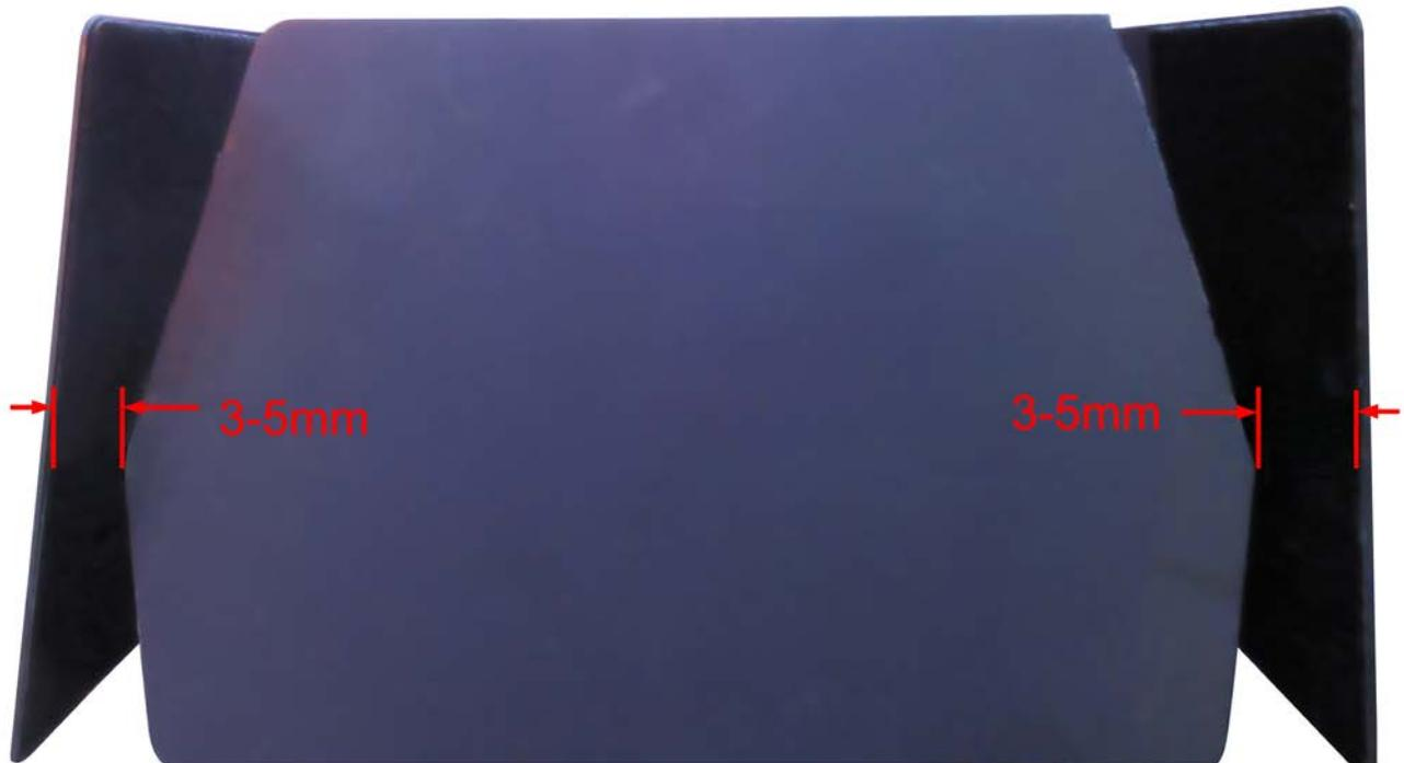
5. If the distance is too small and rubbing occurs, set the large blade console DMX value to 0. Then, adjust the calibration values of Barndoor1 and Barndoor2 to 10 and repeat the above steps to recalibrate the distance between the blades.
