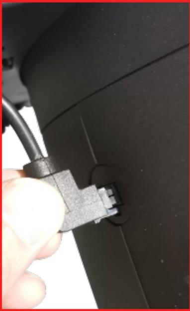
6. To disconnect the Power/Data Connector, depress the toggle-lock to disengage it, and with a firm grasp of the connector body, pull connector straight from socket. Follow steps in reverse order to remove the Barndoor.
