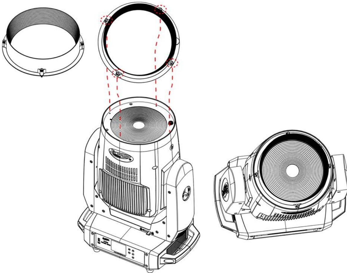
To install either the Beam Shaper or Barndoor, it will be necessary to remove the Snoot.
