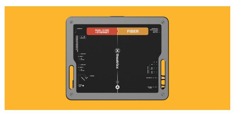
This video converter revolutionises video transmission by converting two 12G-SDI signals into fiber, ensuring high-quality video transmission over extended distances. It also featured two 1Gbps PoE++ ports. This all-in-one solution offers a streamlined and reliable approach to managing video and data management, enhancing your setup's efficiency.
