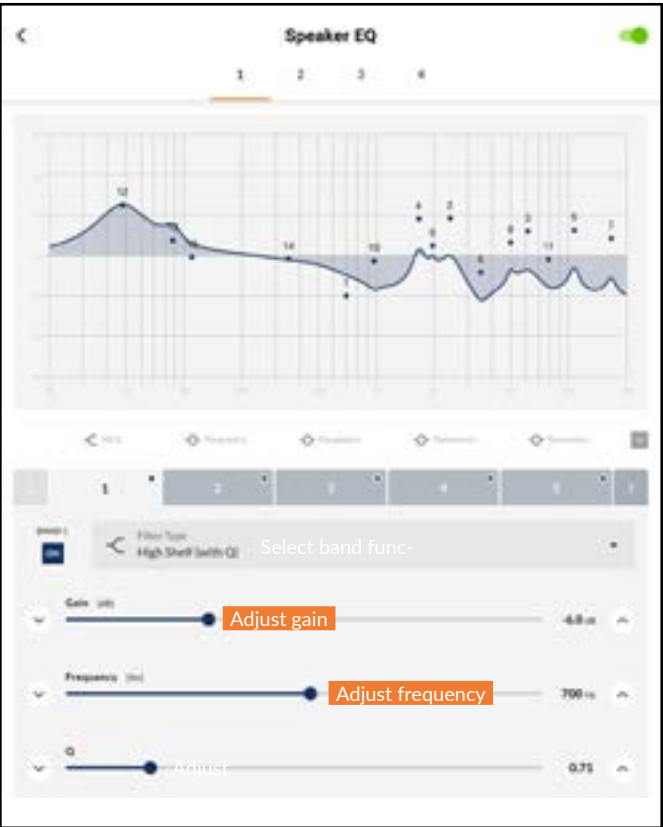
Diagram 6L Speaker Preset parameter adjustment
